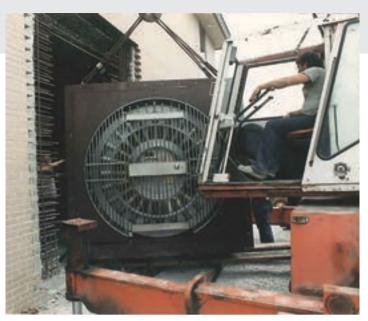
**Figure 22.** Everything that could possibly rattle loose on the truck ride to the new location had to be removed and crated separately.
